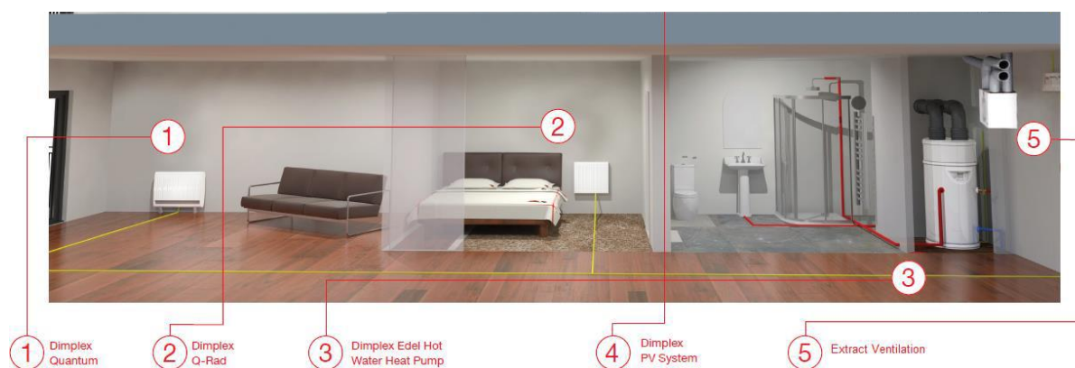
Figure 6 – Air-Source Heat Pump with Electric Panel Heaters
