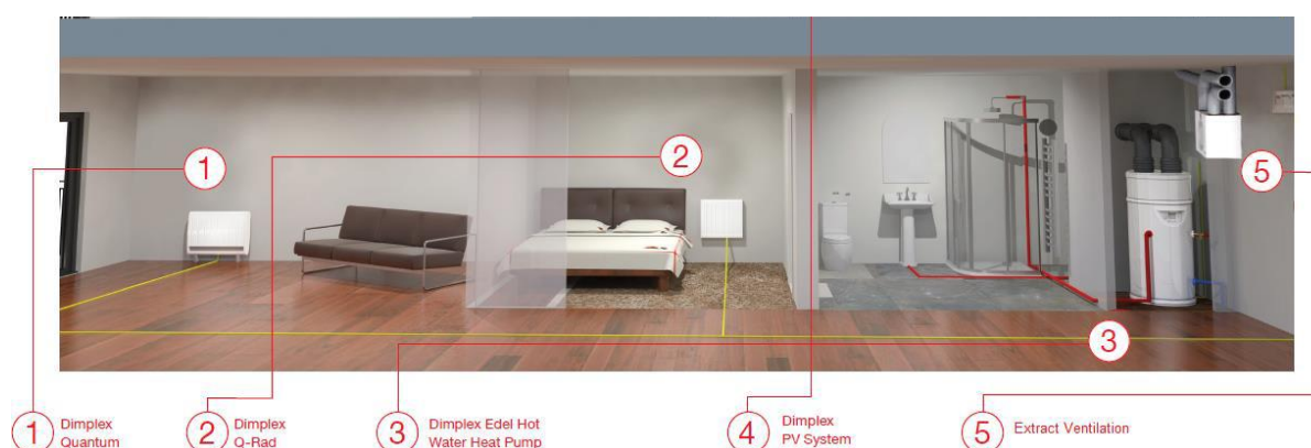
Figure 5 – Air-Source Heat Pump with Electric Panel Heaters
