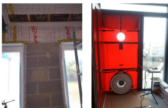
Figure 3 – Air Tightness Testing
